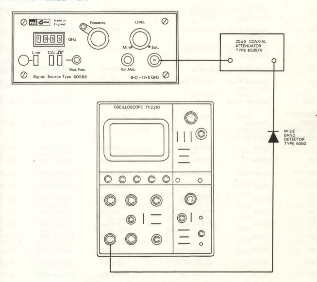
Fig. 12 Modulation Circuit
