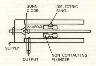
Fig. 6 Microwave Oscillator Schematic
