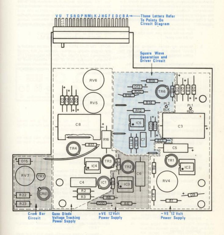
Fig.9 Printed Circuit Board
