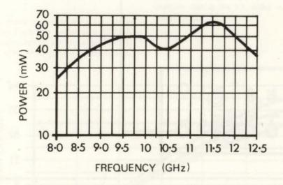
Fig. 3 Output Power As A Function Of Frequency
