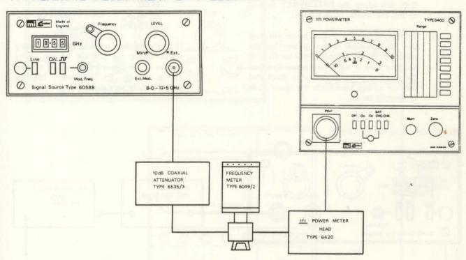
Fig. 10 Frequency Calibration Circuit
