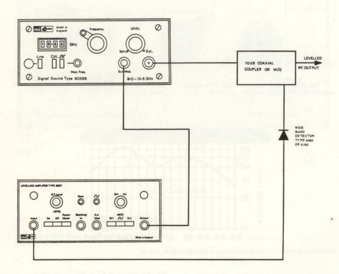
Fig. 4 Levelling Circuit With Type 6587 Levelling Amplifier
