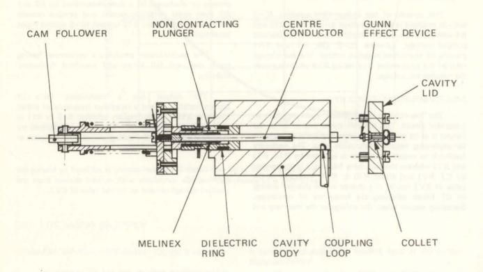
Fig. 8 Cavity Assembly
