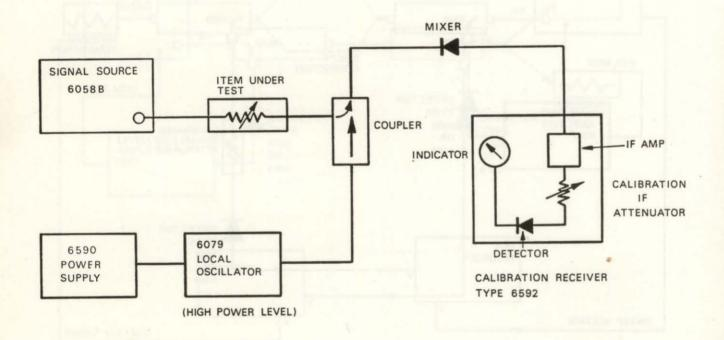
Fig. C1 High Attenuation Measurement
