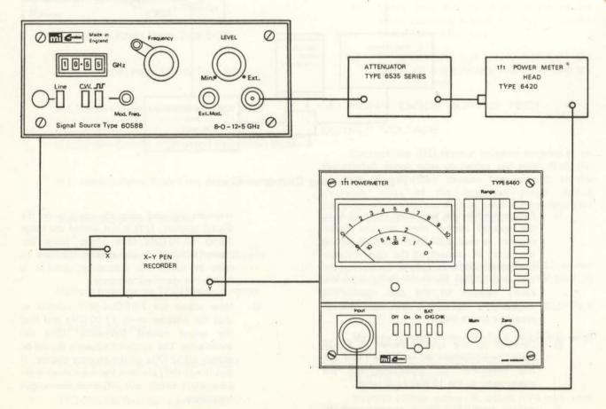
Fig. 11 Attenuation Calibration Circuit
