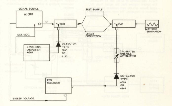
Fig. B1 Transmission Loss Measurements
